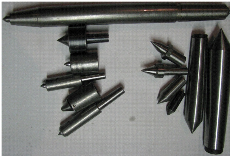
Collection of lathe centers for different lathes and of different styles. Drawings will be described later for making some of these. To the left live centers; right dead centers. Most of these are self-made or came together with the lathe. One is from Sherline, some came with a SIEG lathe.
